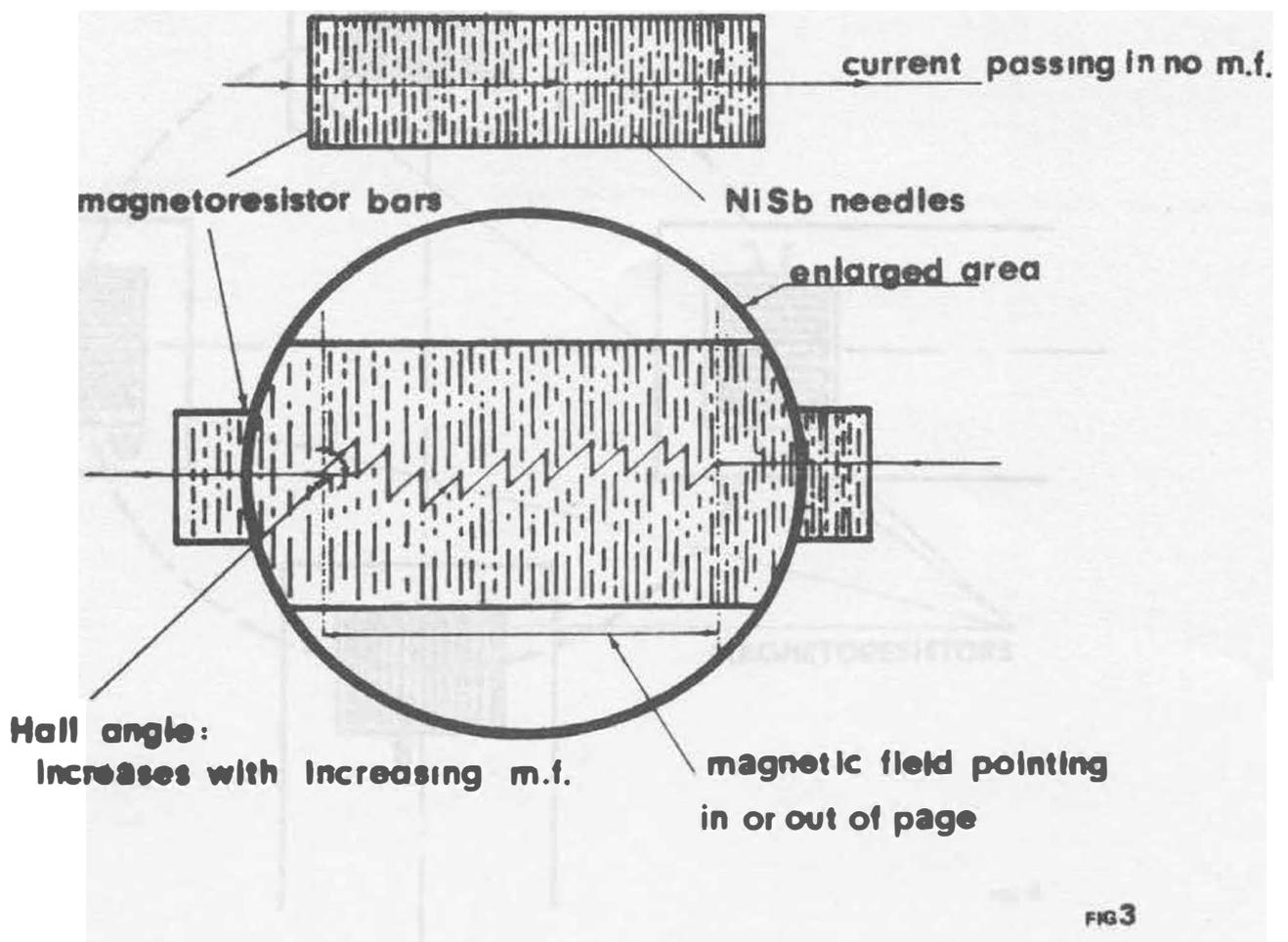
Operating principle of a magnetoresistor (m.f. stands for "magnetic field").
