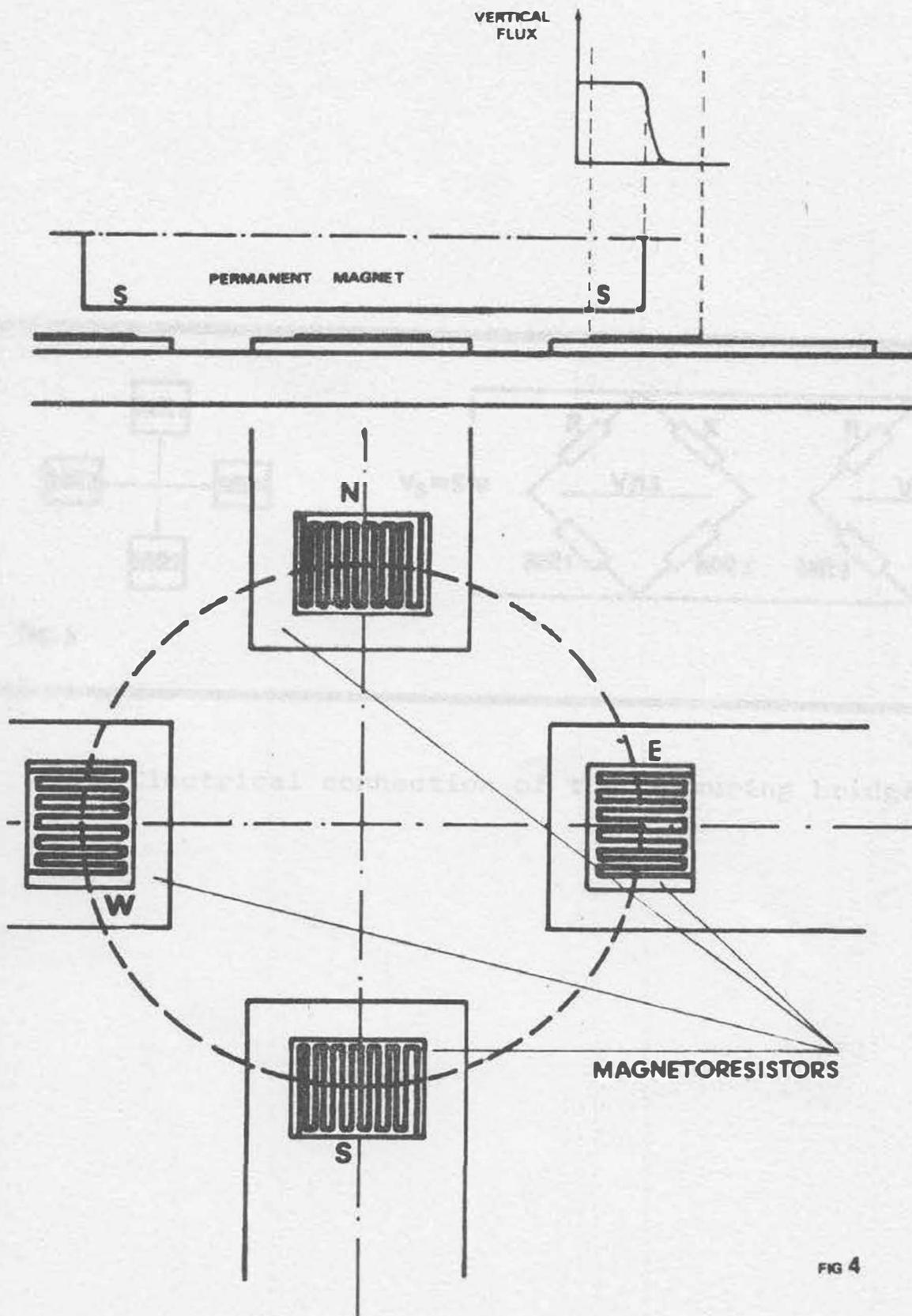
Alignment of sensors below the permanent magnet. The upper section of the figure shows the spatial arrangement of sensors and permanent magnet the change of the vertical magnetic flux is indicated on the diagram in the upper right corner of the picture. The lower part of the figure shows the arrangement of the measuring bridges.
