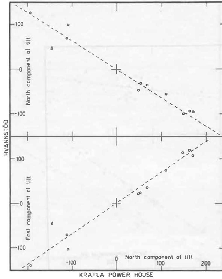
Fig. 6. North and east components of tilt at the tilt station Hvannstóð (0090), plotted against the north component of tilt at the Krafla power house. See Fig.2 for explanation.
