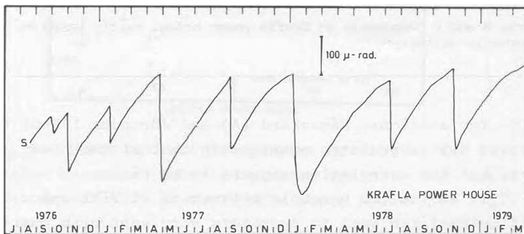
Fig. 7. N-S component of tilt at the Krafla power house based on about two readings every month of the water tube tiltmeter. This and the subsequent four figures are plotted such that the trace is rising if land is rising at the center of tectonic activity in the Krafla region. The letter S at the beginning of the trace means that tilt towards south is up on the graph.
