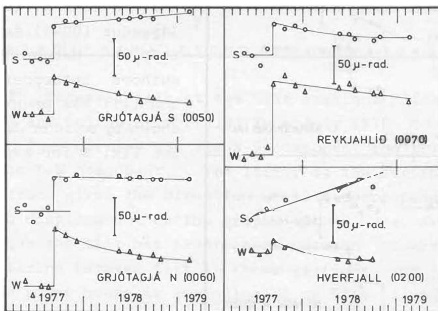
Fig. 11. Observed tilt at the tilt stations Grjótagjá S (0050), Grjótagjá N (0060), Reykjahlíð (0070) and Hverfjall (0200). See Figs. 8 and 10 for explanation.
