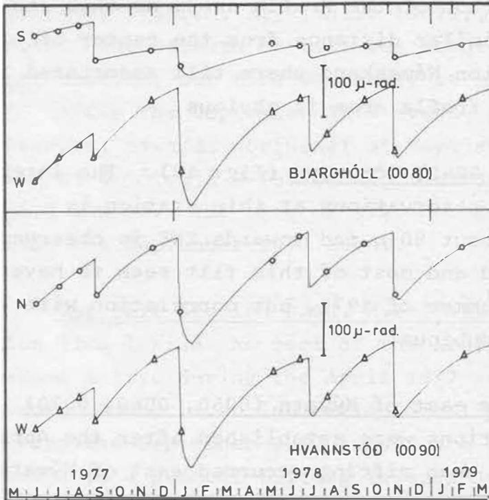
Fig. 9. Observed tilt at the tilt stations Bjarghóll (0080) and Hvannstód (0090) from June 1977 to March 1979. See Fig. 8 for explanation.
