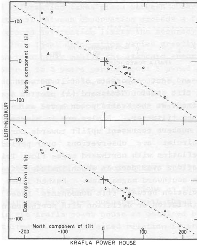
Fig. 4. North and east components of tilt at the tilt station Leirhnjúkur (0010), plotted against the north component of tilt at the Krafla power house. See Fig.2 for explanation
