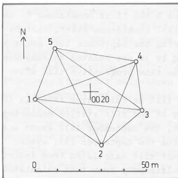
Fig. III,1. The benchmark array of tilt station 0020, Mývatn N.
