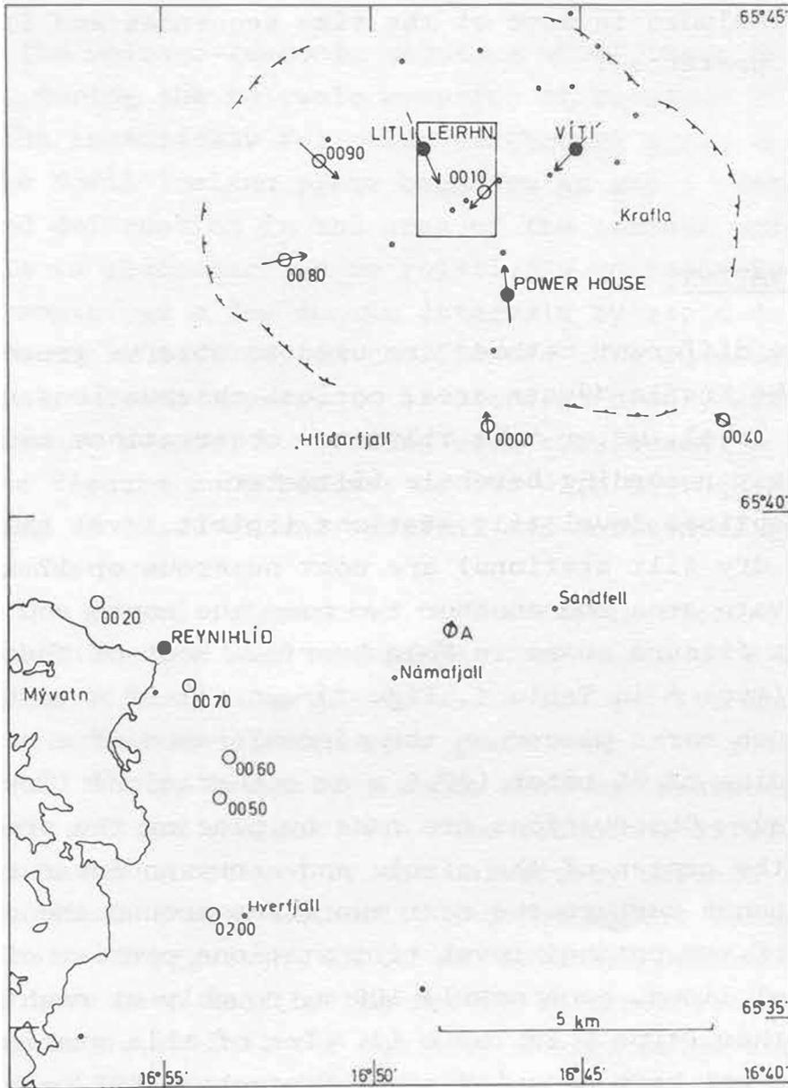
Fig. 1. Location of tilt stations in the Krafla-Mývatn area in February, 1979. Open circles are spirit level tilt stations, filled circles are borehole tiltmeters. Arrows show average tilt during inflation-deflation sequences. Rectangle shows the area of map of Fig. 12.
