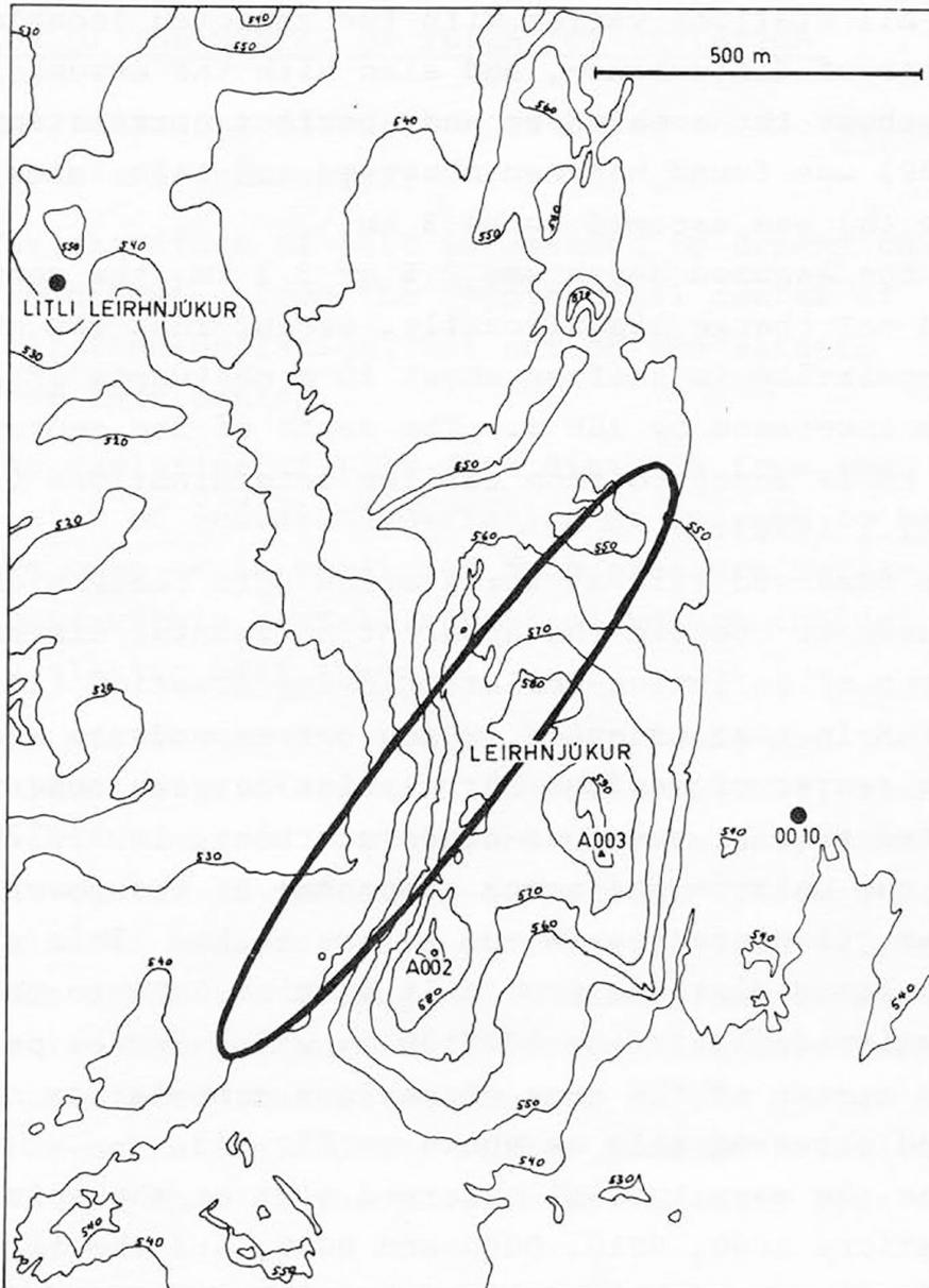
Fig. 12. A map of Leirhnjúkur (see Fig. 1 for location). The correlation between calculated and observed tilt at the stations 0000, 0080, 0090, and the power house is better than 0.99, if center of inflation-deflation lies at 3 km depth below the encircled area, but poorer correlation is found outside this elliptical area.
