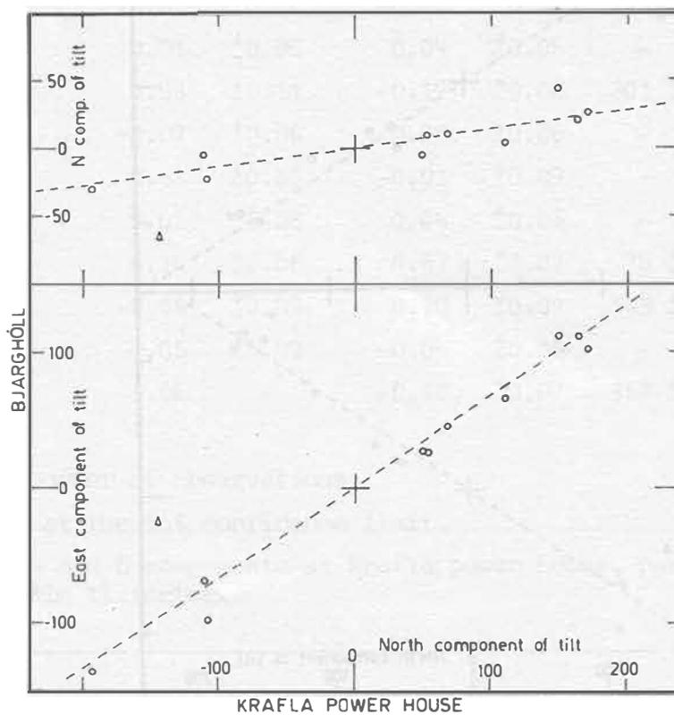
Fig. 5. North and east components of tilt at the tilt station Bjarghóll (0080), plotted against the north component of tilt at the Krafla power house. See Fig.2 for explanation.
