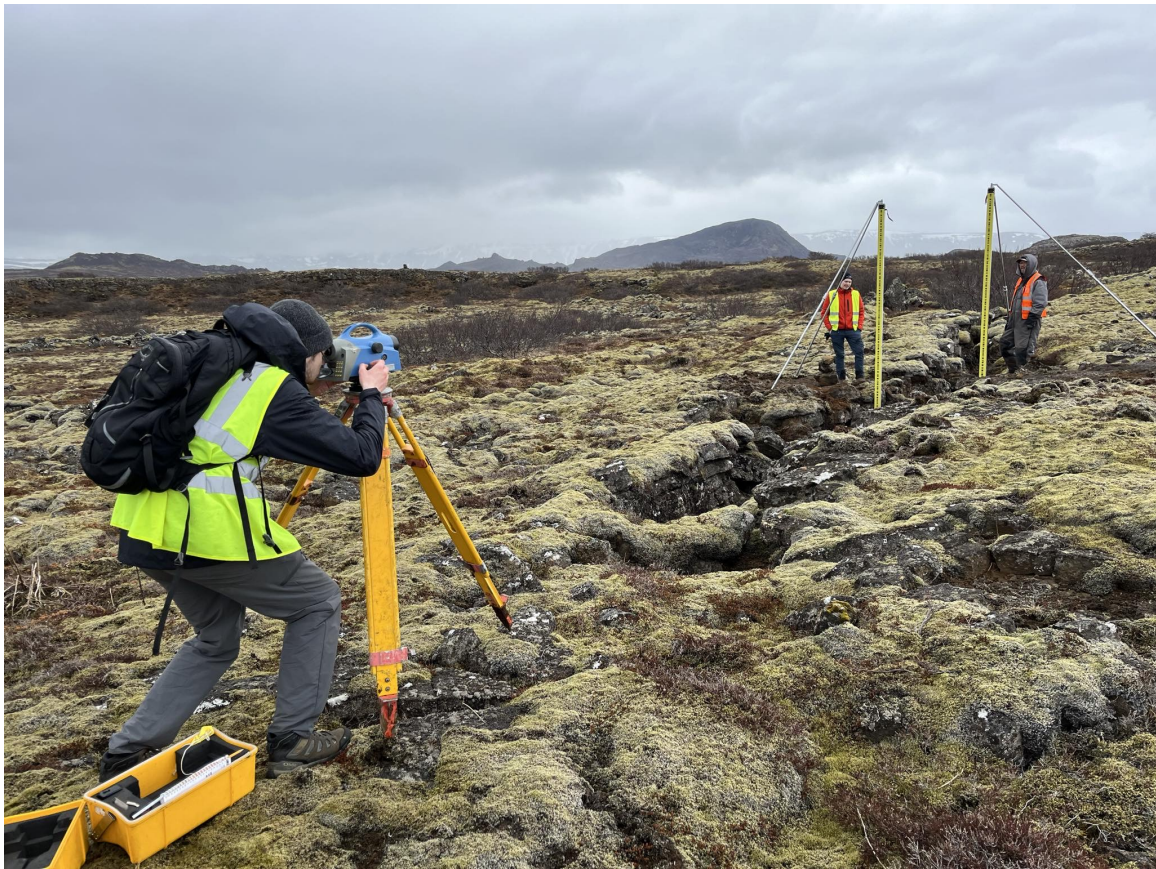
Figure 2: Leveling fieldwork in May 2024. The benchmarks in this image span a fracture.
