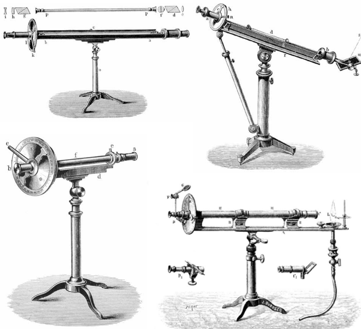
Figure 13-5. Some of the first generation of polarimeters in common use. Top left : The polarimeter of Robiquet (1856), containing two Nicol prisms and a double quartz plate f . From Landolt (1898). Right : A picture from Lummer (1909) of Biot's (1840a) polarimeter with a glass-mirror polarizer and an Iceland spar prism. d is a sample tube. Bottom left : Biot's polarimeter as improved by E. Mitscherlich (1844), with two Nicol prisms. From Landolt (1898). Right : A polarimeter produced by the Soleil workshop from 1846. The picture is from a Duboscq catalog.
