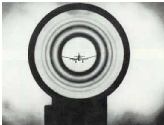
Figure 39-6. Polaroid Corp.'s Optical Ring Sight from World War II. Left: A drawing of its composition. Right: Taking aim at an aircraft. The rings followed the eye of the gunner so that it did not have to be directly over the center of the sight (Wood 1977). The diameter of the device was 3-4 cm and its thickness about 0.5 cm (L. Hughes, pers. comm. 2001).
