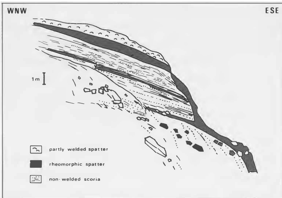
Fig. 6.6. Two welded units joined together forming a rheomorphic flow on the western rim of Eldgjá. Between the spatter units lies a thick non-welded scoria unit containing abundant lithic fragments.
