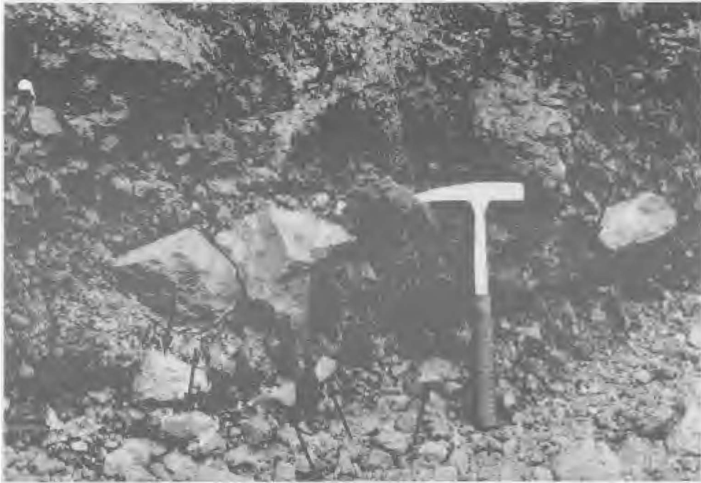
Fig. 6. Layer D, Section I, non-welded scoria with abundant lithic fragments consisting both of dark grey, densely welded material (large fragments) and of pillow lava fragments (arrows).
