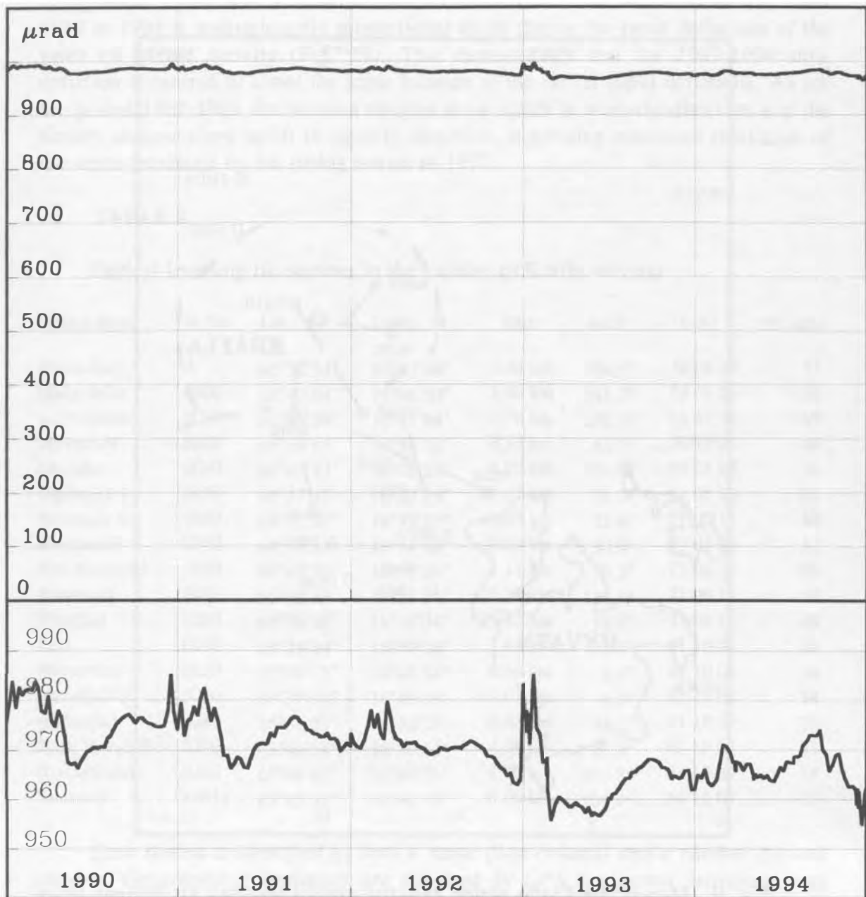
Fig. 8. Record of the north component of electronic tiltmeter at the Krafla power station January 1990 to December 1994. Top diagram is continuation of Fig. 7 in same tilt scale. Bottom diagram is the same record in expanded tilt scale to emphasize disturbances which occur while the ground is frozen, and also temperature effect causing small peaks in late summer coinciding with maximum temperature in the underground cellar where the tiltmeter is located.
