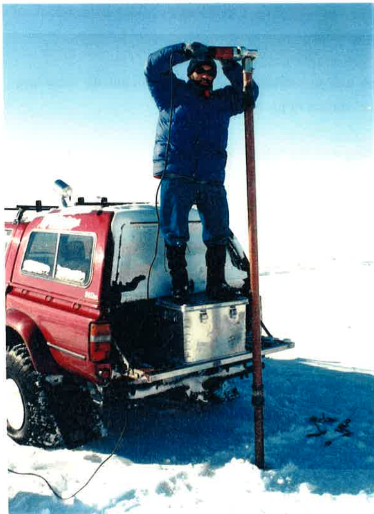
Figure 2. PICO lightweight hand coring auger driven by a Honda generator was used to drill exploratory holes, at the corners of a 40 m by 40 m square corresponding to sites 1, 3, 5, and 7 on fig. 1.
