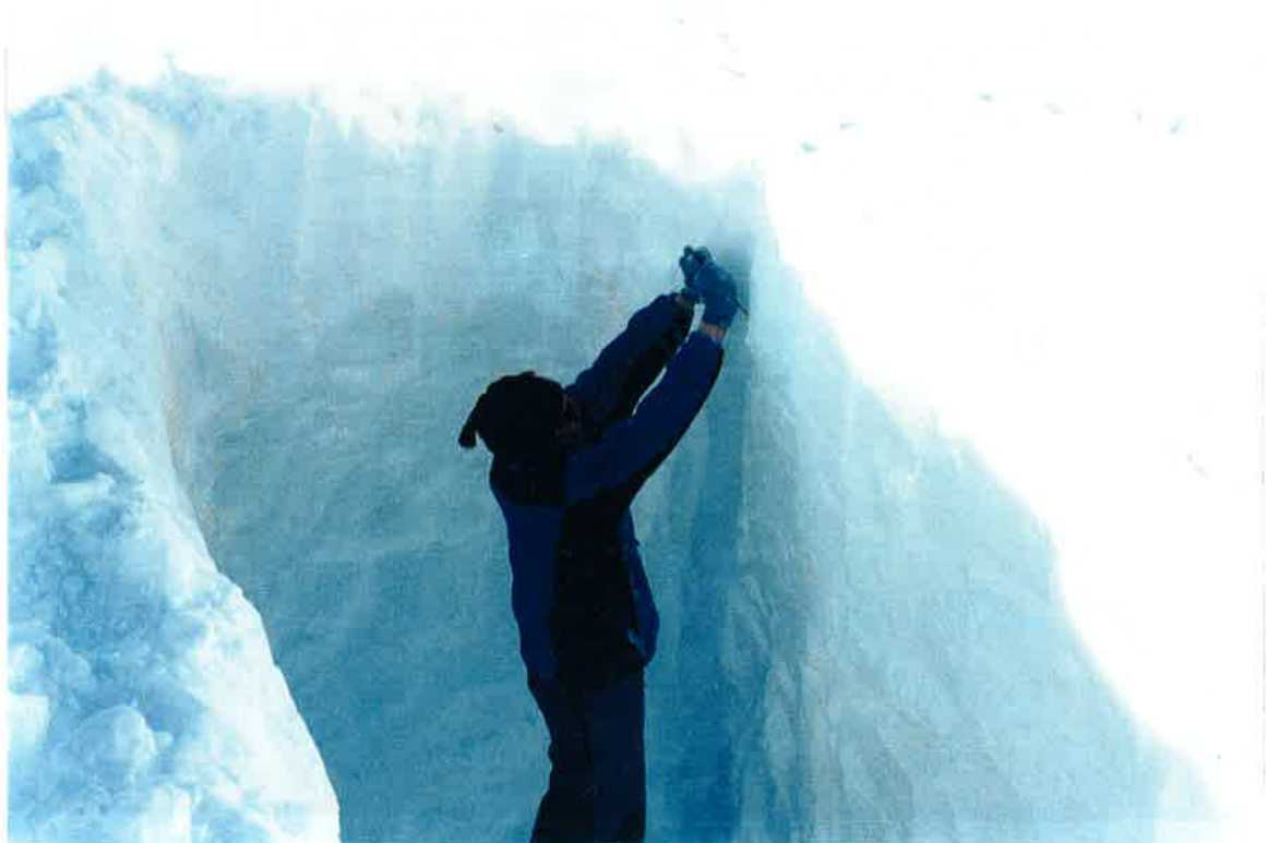
Figure 8. Cleaning the face of the wall with the PC plate, wearing plastic gloves.
